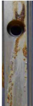
HIRES rail (unloaded) after 32 hours salt spray test (according to DIN EN ISO 9227)
