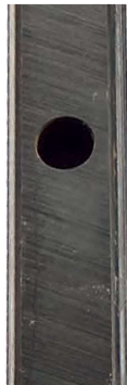
Rail (unloaded) with CCB coating - after 24 hours of salt spray test (according to DIN EN ISO 9227)
