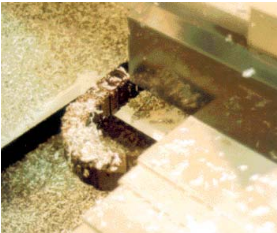
E2 E-Tubes mounted unsupported and on the side in a chip area
