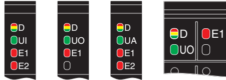
Figure 10-2 LEDs on the power connectors (examples)
